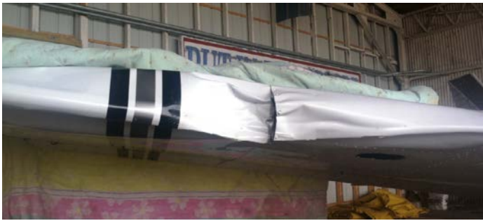
A PA-28 aircraft struck a Canada goose at 50 feet AGL on final approach to a GA airport in the upper Midwest on 21 April 2014. The aircraft sustained substantial damage to the wing and was out of service 720 hours for repairs. Canada goose strikes with civil aircraft have declined from a peak of 87 reported in 1998 to 57 in 2014. Photo by aircraft owner.
