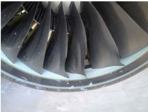
An Airbus 319 ingested a red-tailed hawk in the #1 engine during the take-off run from a southern U.S. airport, August 2014. The pilot aborted take-off at 143 knots. Aircraft was out of service 120 hours; cost of engine replacement and other repairs was $6.5 million. Red-tails are the hawk species most frequently struck by civil aircraft in USA (Table 17). Photo, aircraft operator.
