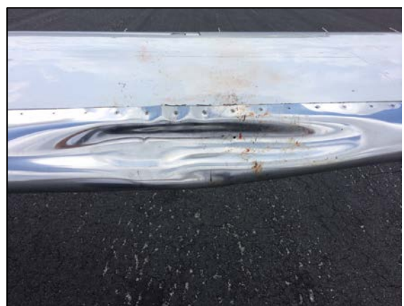
A Cessna 560 struck a turkey vulture at 1600 feet AGL on approach to a general aviation airport in Florida, July 2014. The leading edge of wing and deicing unit were damaged. Repair costs were $162,000 and aircraft was out of service for 2 months. Photo by aircraft owner.
