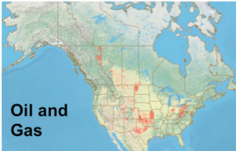
FIGURE 3.7 U.S. CO 2 sequestration capacity estimates for various geological reservoirs. Saline aquifers have the highest potential for CO 2 sequestration, followed by depleted coal beds and oil and gas fields. SOURCE: Created using NATCARB, http://www.natcarbviewer.com/ .
